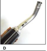
Assemble the silencers with their respective final bodies (Fig. A - D) fix them with the springs in the pack (Fig. B - E); position the 2 metal bands (in the pack) without tightening the screws (Fig.C - F); the right hand final body is the shortest of the 2:
